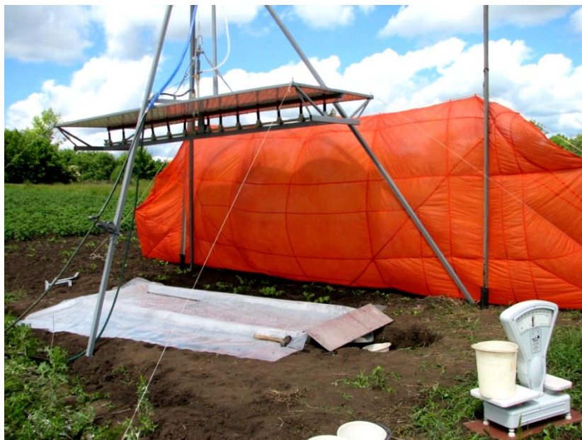
Fig. 1. The large rainfall simulator in the runoff plot 3 m 2 long.
