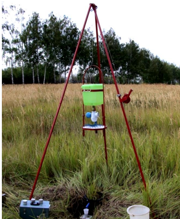
Fig. 2. The portable rainfall simulator in the area of runoff plot of 0.05m 2 .
