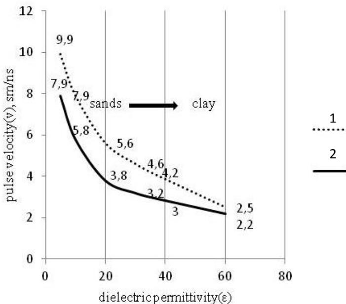
**Fig 1.** Changes in the impulse speed and dielectrical permeability of grounds with varying particle-size distribution for moisture categories (1 – maximal hygroscopic water; 2 – minimum field capacity).
