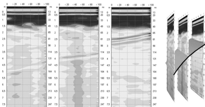
**Fig. 3.** The surface of local object at the territory of the cutting steppe in Central biosphere reservation (the Kursk region) identified by synphasic axes of georadar profiling.
