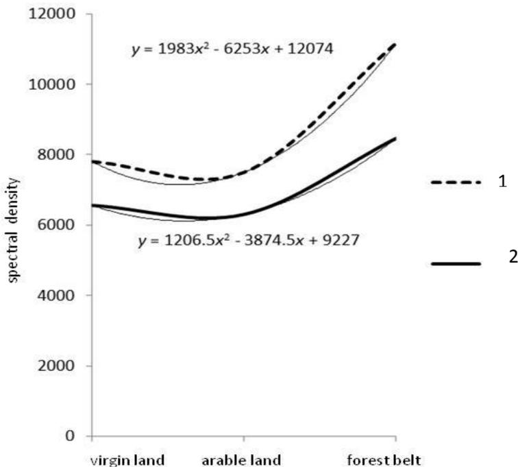
**Fig. 5.** Changes in average values of spectral density of reflected impulses along the ways of georadar profiling of chernozems (1 – ordinary chernozem, Voronezh region; 2 – typical chernozem, Kursk region)
