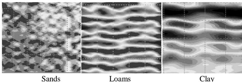
**Fig. 2.** Visualization of parameters for reflected impulses, characterized the grounds with different particle-size distribution.
