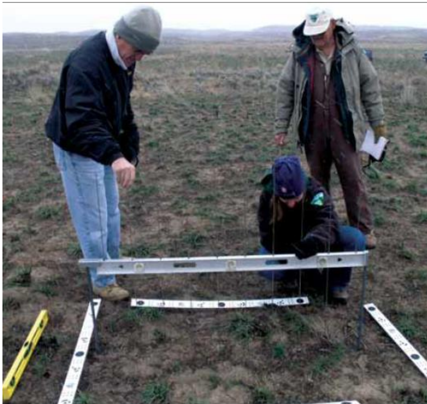
Fig. 1. Erosion bridge used for quantitative assessment of wind erosion intensity in a burned-out area, 2 years after the fire, Idaho (USA) ( Ypsilantis, 2011 ).
