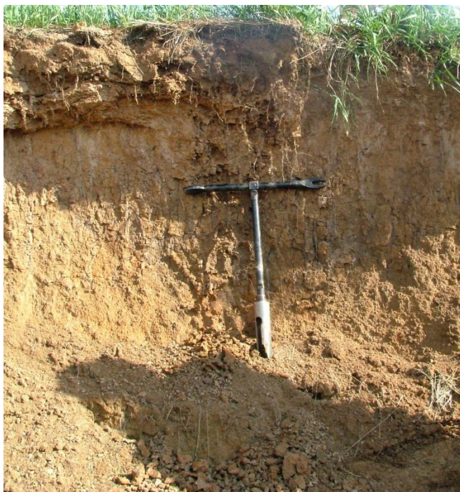
Fig. 1. The typical profile of quasizem – technogenic surface formation (flying airfield “Domodedovo” in the Moscow region).
