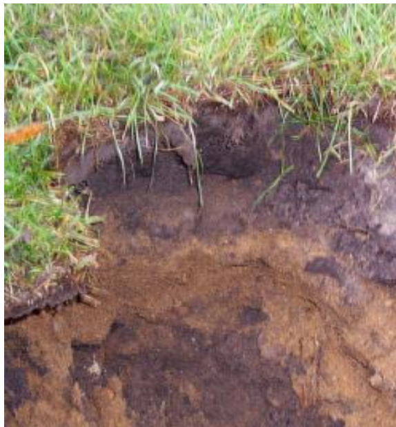
Fig. 2. The morphological profile form of primitive quasizem (pit 2-ИЗ-06; the football ground “Spartak” in the Moscow region).
