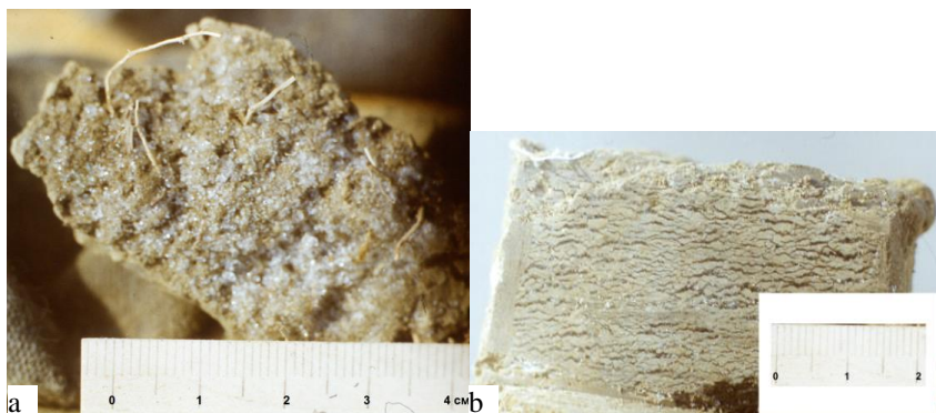
Fig. 1. The structure of frozen profile of Cryosol: a – the A 1 horizon; b – the CR horizon.
