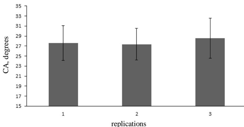
**Fig. 2.** Contact angle of kaolinite mineral. Standard deviation is calculated for 7 analytical replications. Measured on sticky tape.
