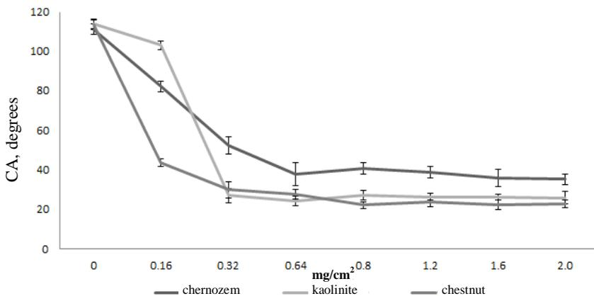
**Fig. 4.** Contact angle for different concentrations of kaolinite, chernozem and agro-chestnut soil. The mean values with standard deviations are shown. Measured on membrane filters.
