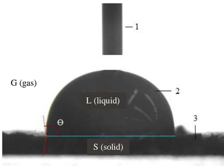
**Fig. 1.** Determination of contact angle. 1 – needle for drop delivery; 2 – a drop of liquid; 3 – the test sample;  $\theta$  – contact (wetting) angle.
