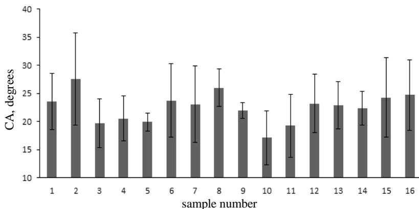
**Fig. 3.** Contact angle of agro-chestnut soil. Standard deviation is calculated for 7 analytical replications. Measured on sticky tape.
