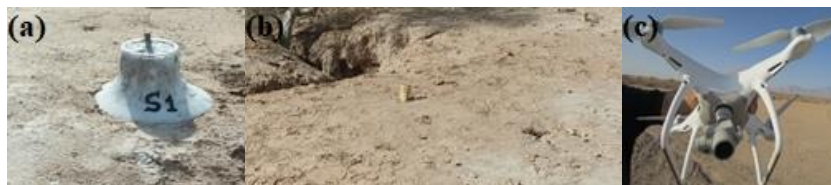
Fig. 3. A concrete station as standard point (a), index points (b) for measuring by level detector and Phantom 4 drone for high resolution imagery (c).
