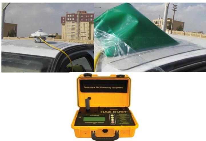
Fig. 1. Pyranometer installation on the car and the used Haz-Dust instrument.
